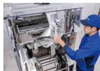
Forming tube side loading system
