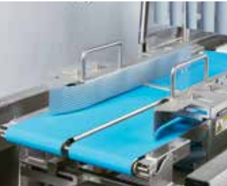
Spacing conveyor with motorised infeed guides
