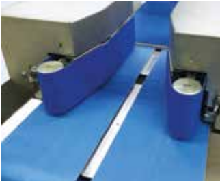
Self-adjusting side belts
