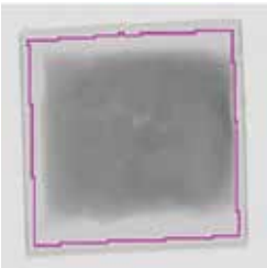
Masks packaging on product to enhance foreign body detection
